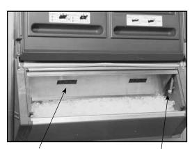
Safely loosen congealed ice **through** SmartGATE ice shield with optional ice paddle accessory. Released ice remains **behind** SmartGATE ice shield.
